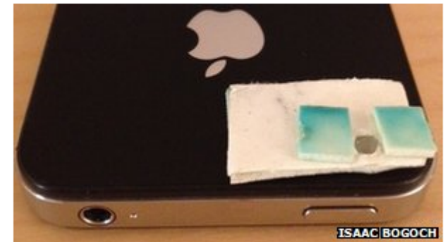
Slides were stuck to the lens with double sided tape and lit with a cheap torch
